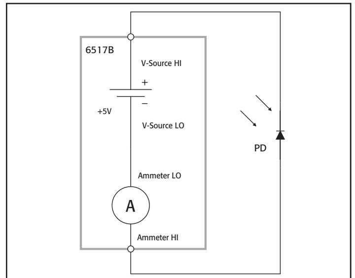
Figure 3b. LED Source Circuit
