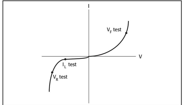
**Figure 1. Typical LED DC I-V Curve and Test Points (Not to Scale)**
