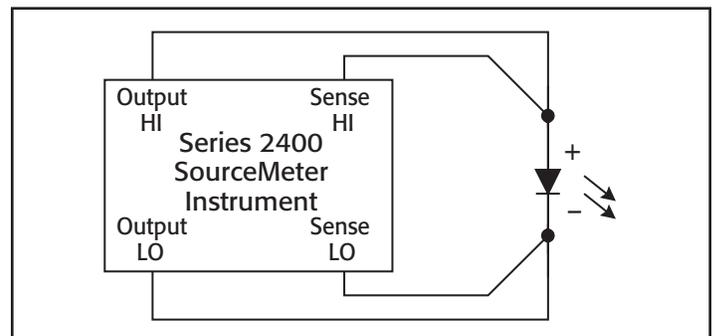
Figure 6b. Four-Wire Connection
