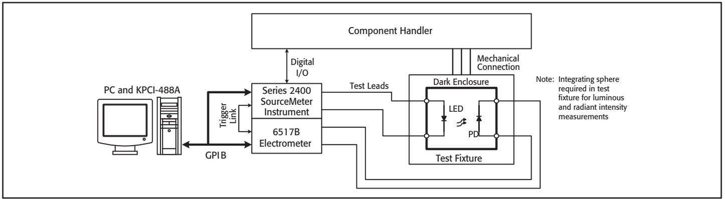
Figure 2. Block diagram of a typical SourceMeter®/electrometer-based test system for visible LED production testing
