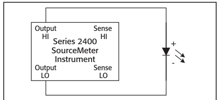
Figure 6a. Two-Wire Connection
