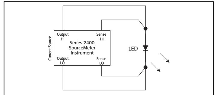
Figure 3a. Photodetector Measurement Circuit
