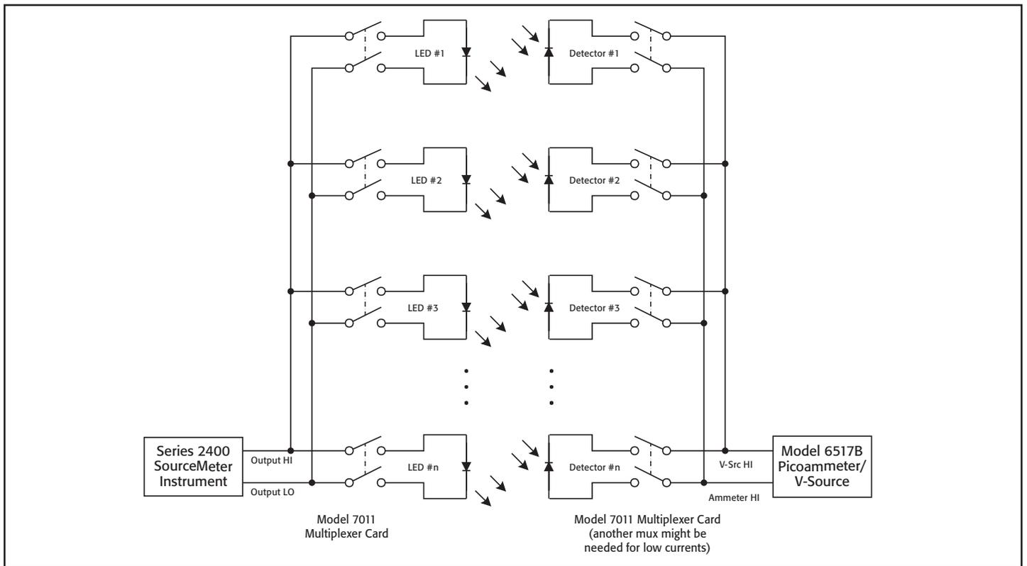
Figure 4. Switching multiple LEDs to a Series 2400 SourceMeter Instrument and PDs to Model 6517B Electrometer
