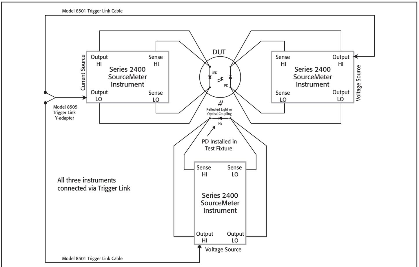
**Figure 5. Measuring an Integrated LED/PD Device with Series 2400 SourceMeter Instruments**
